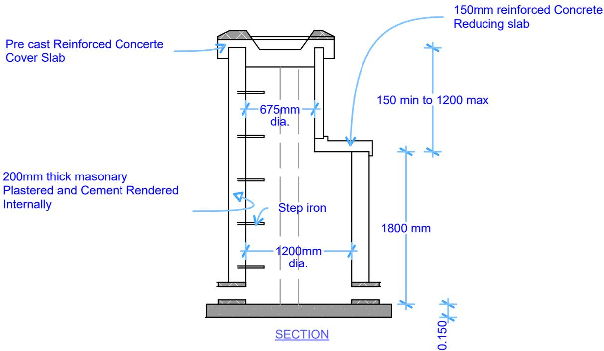
Step iron to BS 1247, staggered 150mm from each side of centerline and spaced @ 300mm vertically
